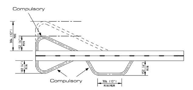
6. A steel wheel guard MUST be fitted around the offside (right) rear wheel, from rear bumper to nerf-rail. The wheel guard MUST be bolted to its mounts at BOTH ends using MINIMUM 10mm high tensile nuts and bolts. Nearside (left) wheel guards are OPTIONAL but MUST be mounted as above.
